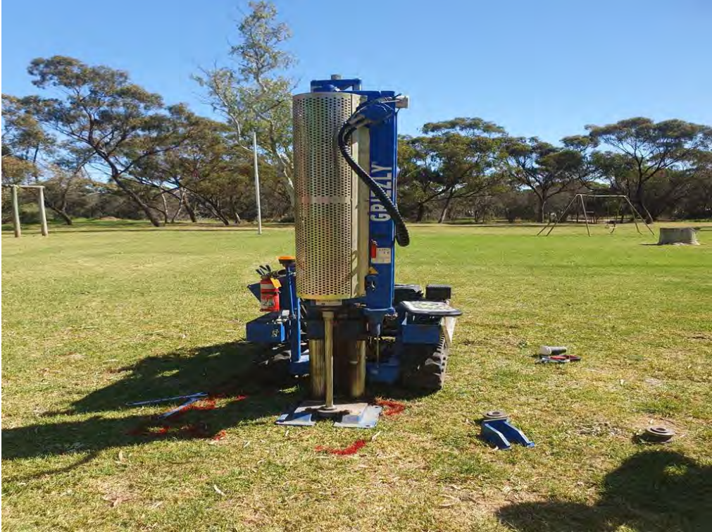
Photograph 5: Facing north, DPSH02 in progress
